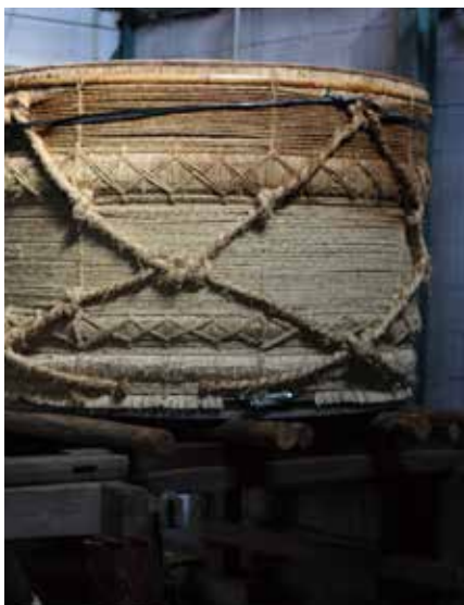
蒸米に使う大型のセイワは木製で、今では作れる職人がほとんどいない特注品。 A large steamer for sake rice is made of wood. It is an order made item since there are so few artisans who can make them now.
